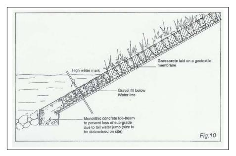
With its traffic bearing capability, GRASSCRETE can be specified as a complete wear layer to reservoir berms with crest access for heavy vehicles being accommodated.
